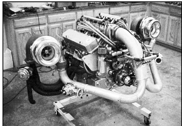
2886 HP Aluminum Pontiac engine in Rodney Butler's GTO. Uses Ferrea Titanium Valves.
