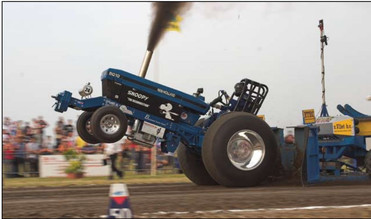
Pro Stock Snoopy, competing in the Dutch Championship Tractor Pulling, with heads by BFS-Holland Martin Wolters uses Ferrea Titanium Intake and Super Alloy Exhaust Valves to run at app. 6000 RPM, reaching 2000° F with boost at least 90 psi. single turbo.
